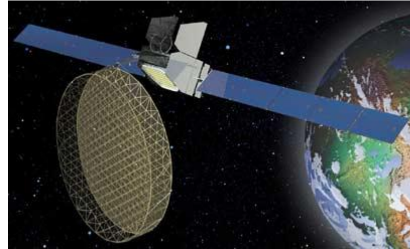
Multiple Spot Beams created from a single AESA antenna
